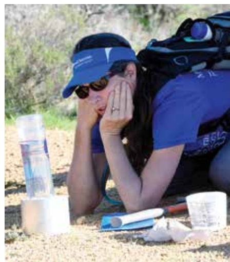
Infiltrimeters, designed by steward Bill Sowle, allowed us to compare water infiltration rates between ripped and unripped soils. Principal investigator Helen Rowe discovered this can be slow business in highly compacted soils. Photo by Tiffany Sprague
